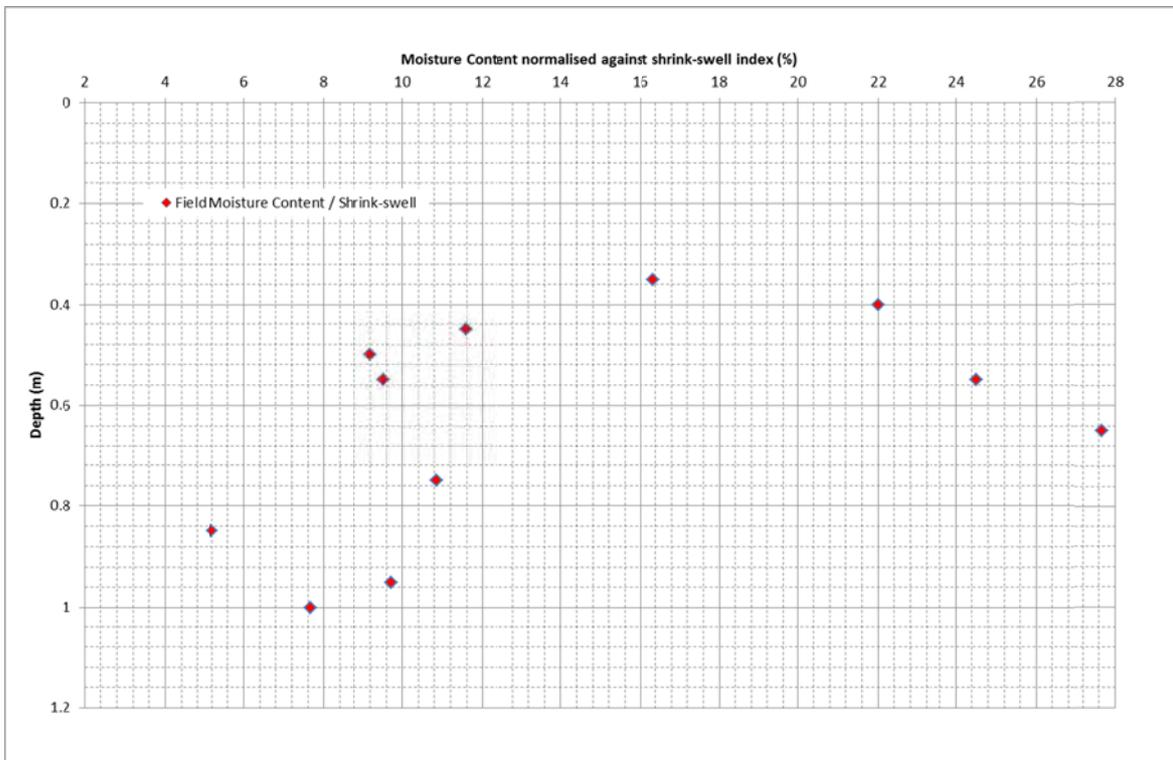
Figure 9: Field moisture content normalised with shrink-swell index against depth
