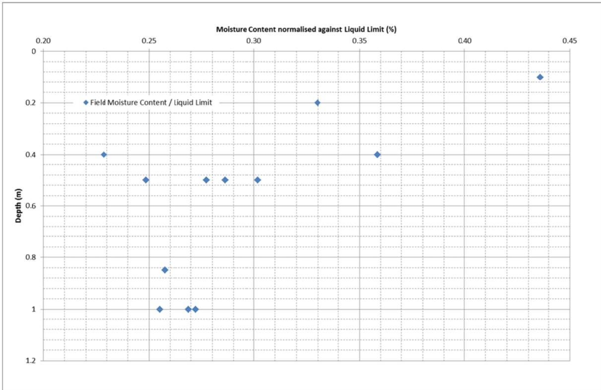
**Figure 7: Field moisture content normalised against liquid limit with depth**
