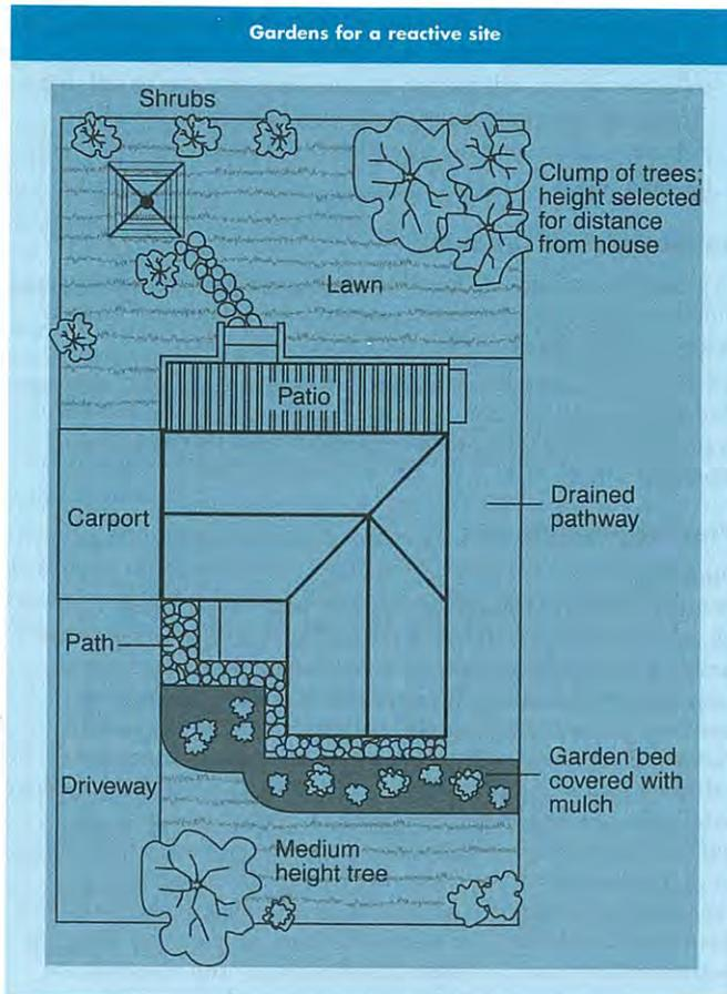
extend outwards a minimum of 900 mm (more in highly reactive soil) and should have a minimum fall away from the building of 1:60. The finished paving should be no less than 100 mm below brick vent bases.
