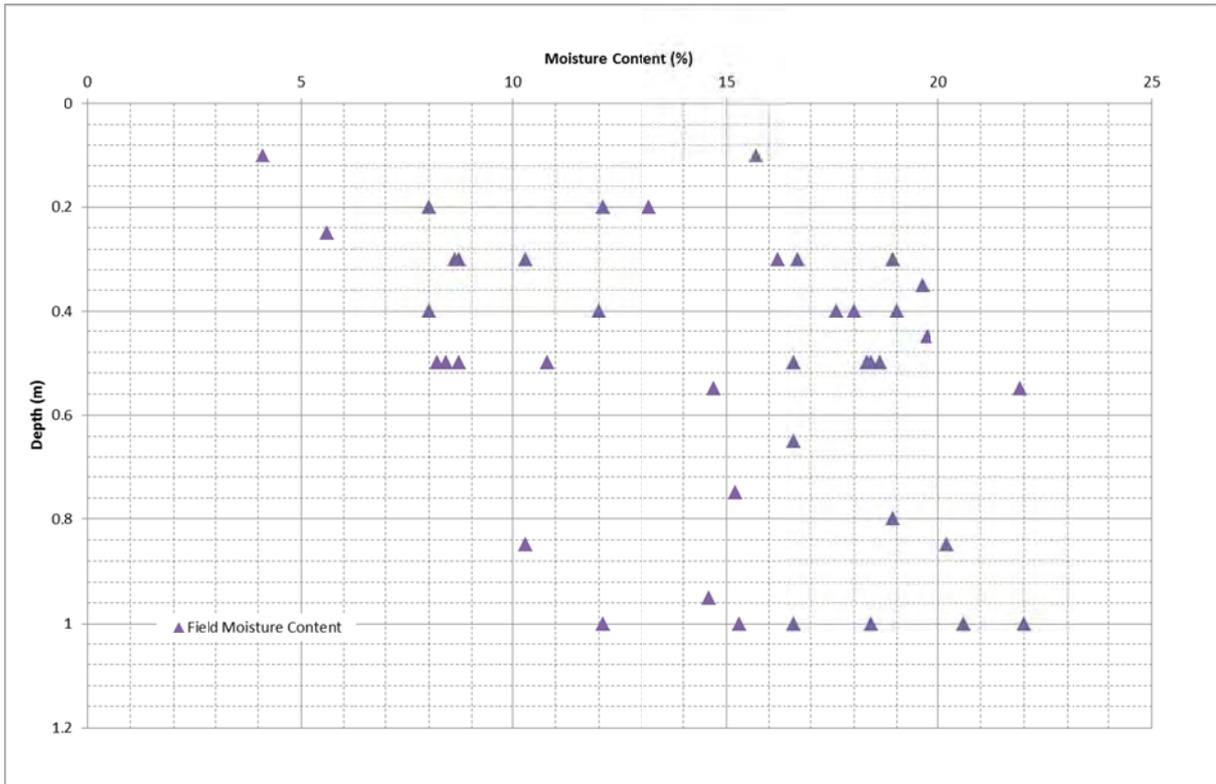
**Figure 6: Field moisture content versus depth of sample**
